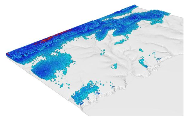
Figure 12: Regions with wind speed above 7m/s (gltf file imported from Paraview)
