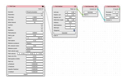
Figure 92: FloVi node setup
