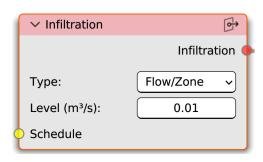
Figure 40: EnVi Infiltration node
