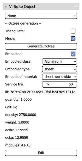
Figure 67: VI-Suite Embodied carbon object properties
