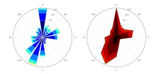
Figure 62: Histogram and contour wind roses
