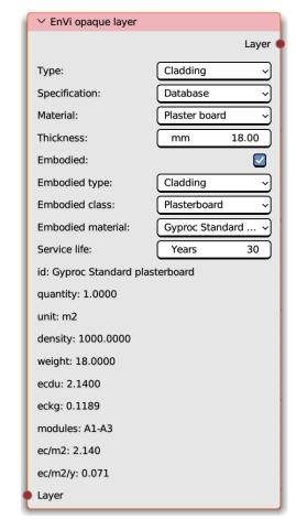
Figure 46: EnVi opaque layer node (18mm plaster board with embodied carbon)
