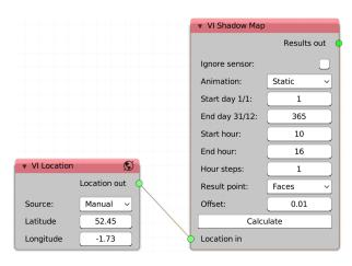
Figure 64: Shadow Map node set-up
