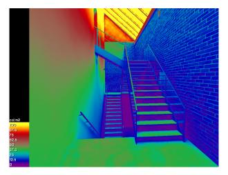
Figure 80: LiVi falsecolour processing showing scene brightness
