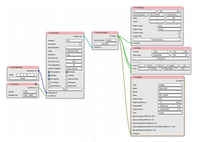
Figure 82: Typical EnVi node set-up with VI Chart, VI Heatmap and VI Metrics visualisation nodes
