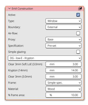
Figure 45: EnVi Construction node
