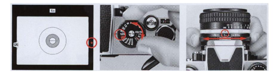
First, position your main subject at the centre of the field of view inside the viewfinder. Then turn the shutter speed dial and/or lens aperture ring until the LED lamp for the symbol for correct exposure O lights up.
