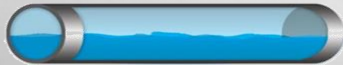
vi) Stratified wavy flow
