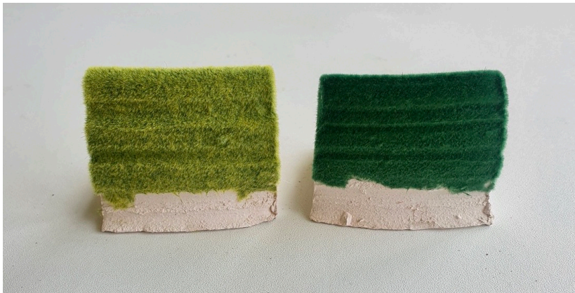
Experiment for a moss like texture with the polymer's technique of flocking.
