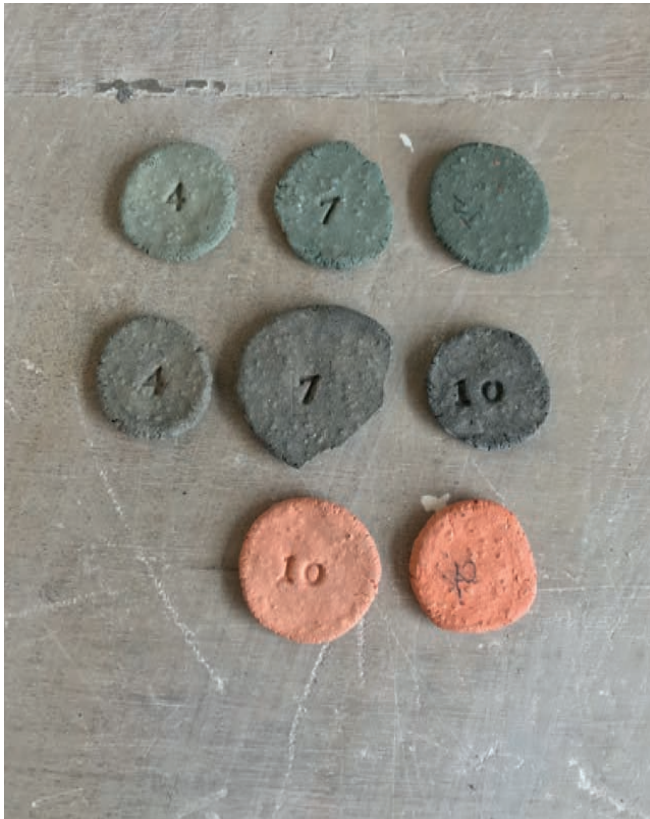
Testing stained crank clay at different percentages
