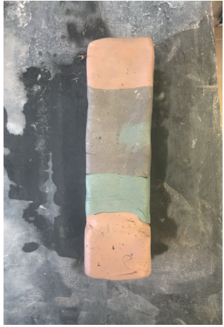
Piling different coloured crank clays into the extruder to get random patterns in the clay body, created from the pressure of the extruder.
