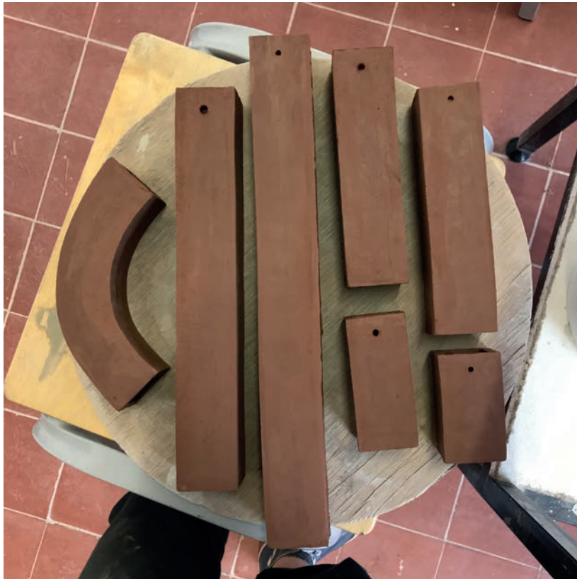
Extruding enabled me to semi batch produce these long chime like pieces which then allowed me to be more ambitious with larger scale installations I eventually made.
