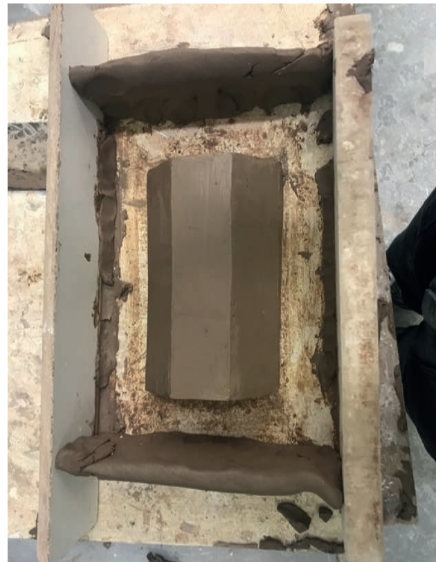
MDF sledging profiles used to create reclaim clay masters
