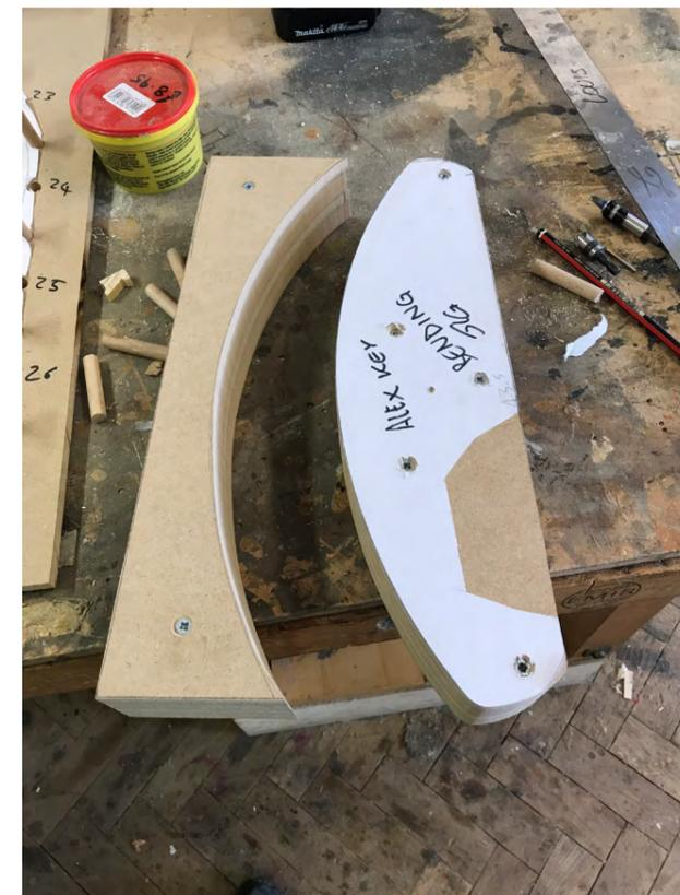
Back block for steam bending JIG
