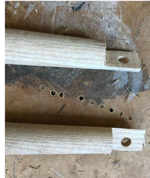
Back joining holes (8mm) in back spindles
