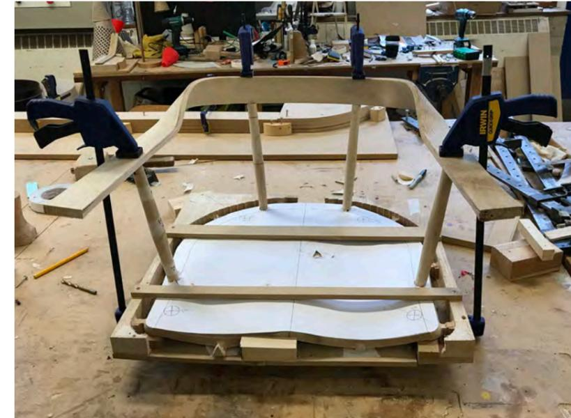
Laminated back dry test attachment to spindles
