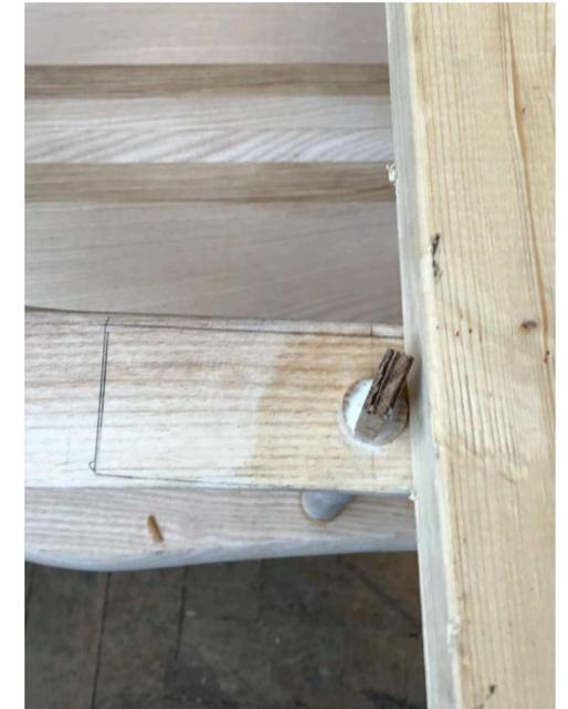
Back attached to front spindles wedged & glued
