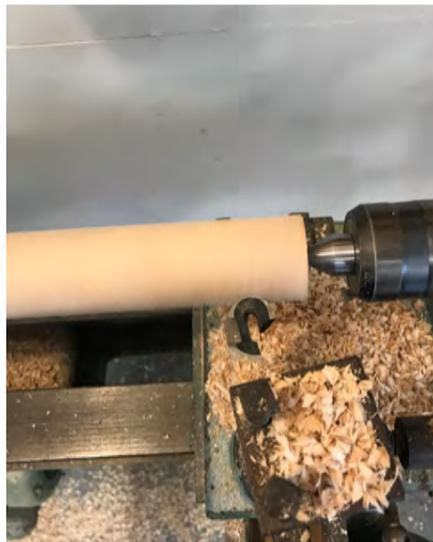
Rounding leg blanks on the lathe
