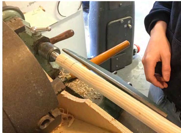
Leg shaping on the lathe using a skew chisel & parting tool
