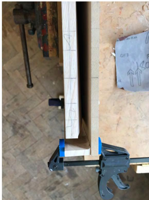
Biscuit cutter markings on joining edge
