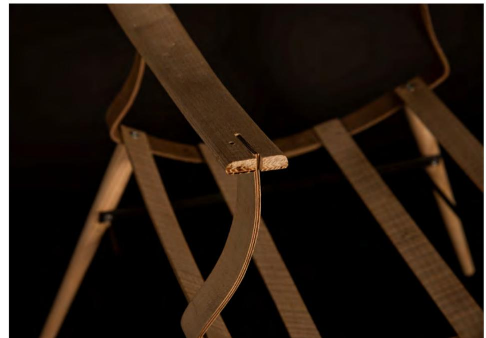
Close up of test back joint to seat frame
