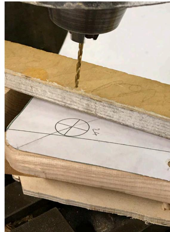
Front leg pilot hole (3mm) being drilled
