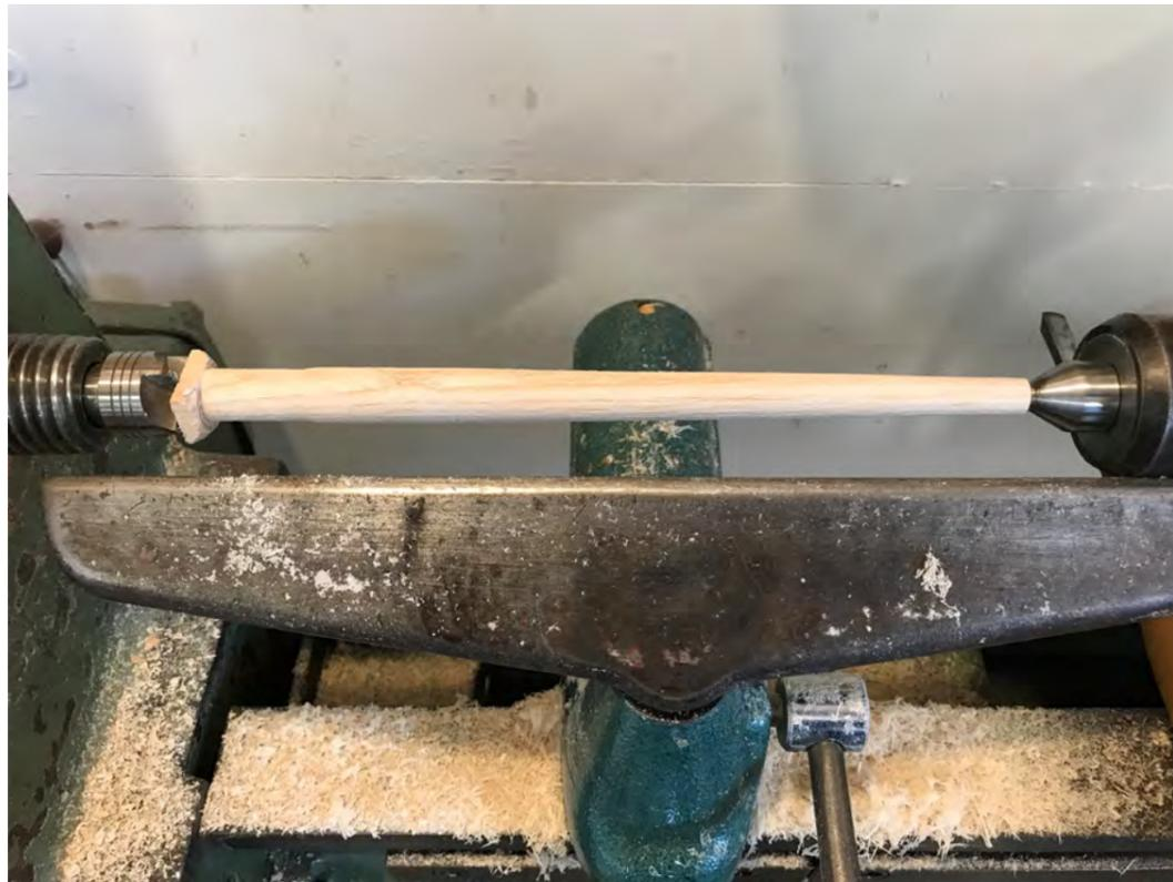
Half-scale sycamore legs on the lathe
