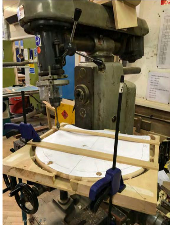
Front leg hole drilling (25mm)
