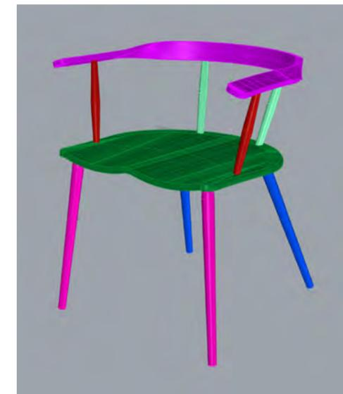
10. Legs, seat, spindles & back assembled
