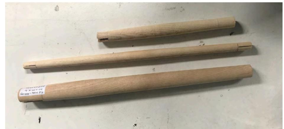
Leg, side & back spindle tests
