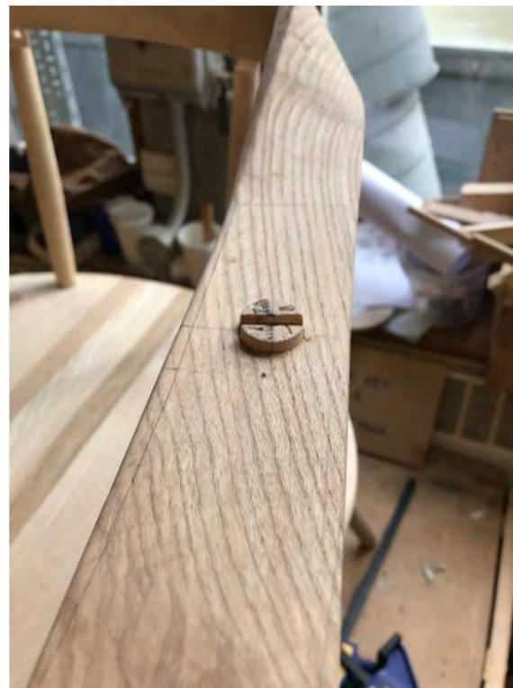
Front spindle wedge joint
