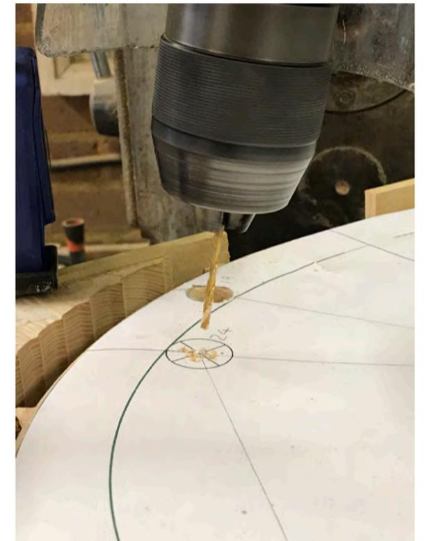
Back leg pilot hole (3mm) being drilled
