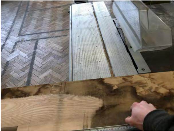
Rough timber being cut up into seat blocks using the table saw
