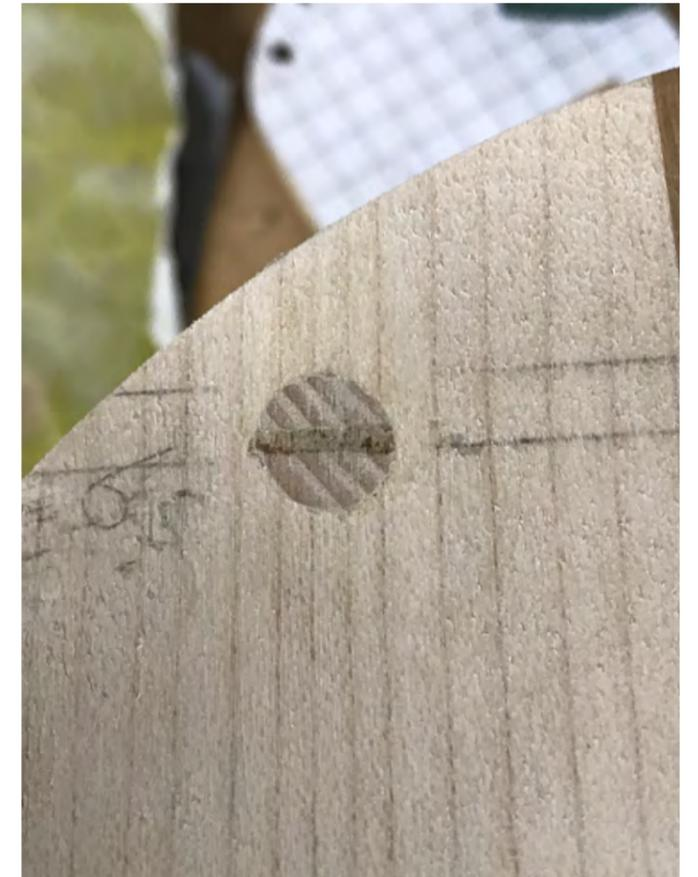
Half-scale leg wedge joint cleaned up
