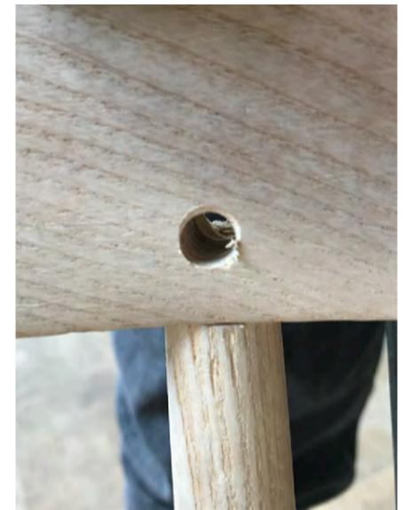
Back joining hole drilled (8mm)
