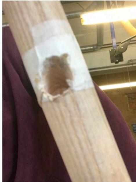
Side spindle lower hole drilled (8mm)
