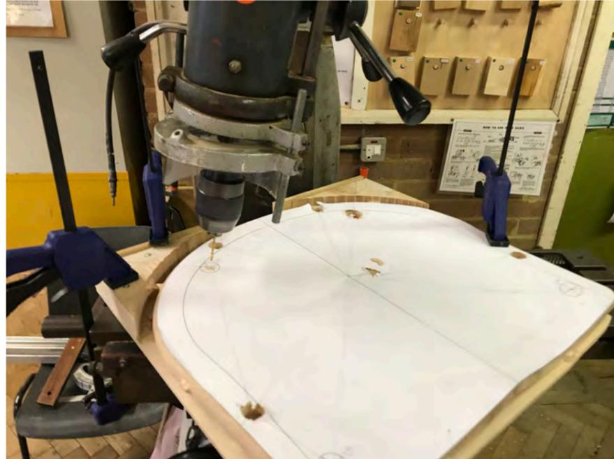
Back leg pilot hole drilling set up
