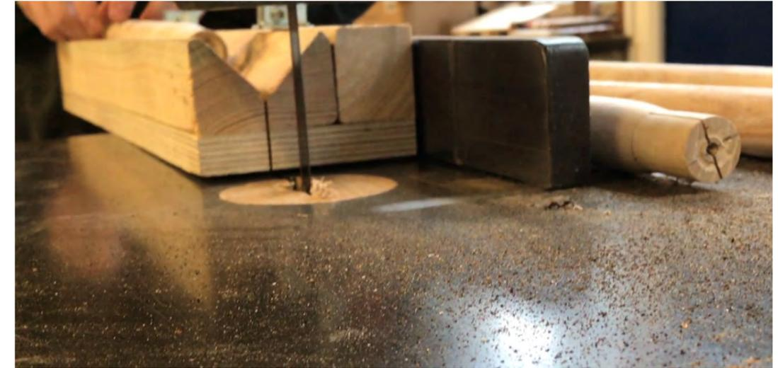
Wedge slot cutting on the bandsaw 1
