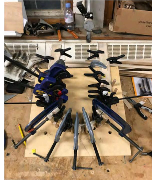
First glue lamination back test - Clamp up A
