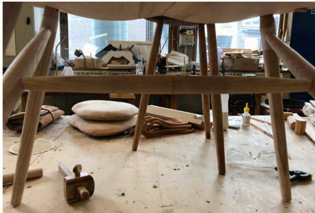
Centre spindle holes drilled & dry assembly
