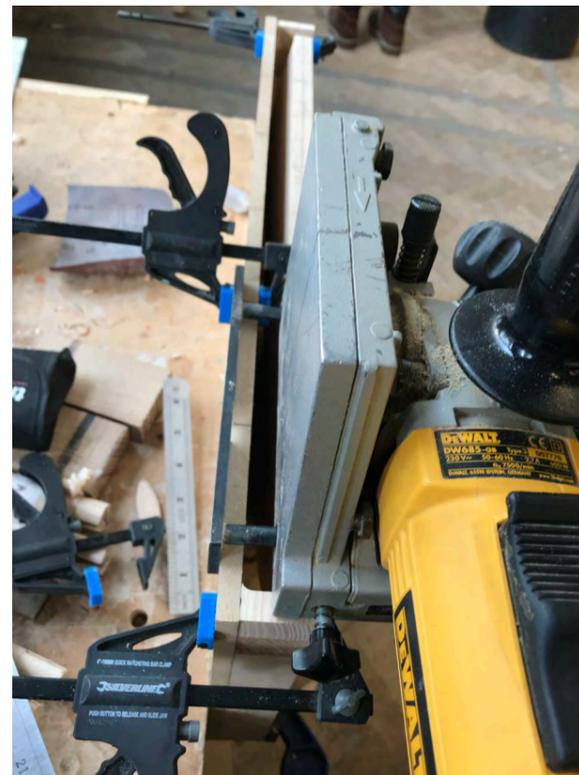
Biscuit cutter set up ready for the first cut
