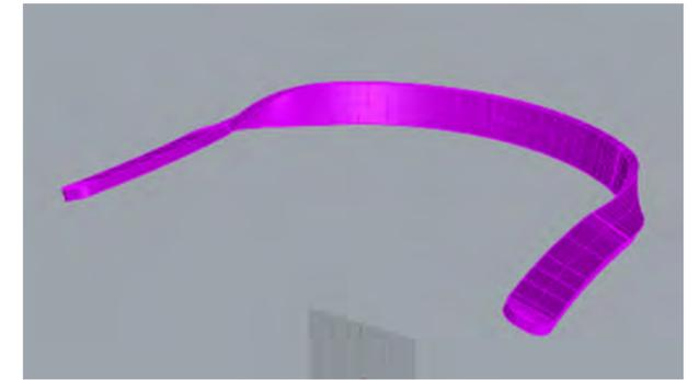
8. Surface applied to back wire frame via creating a surface from 2,3,4 edge curves
