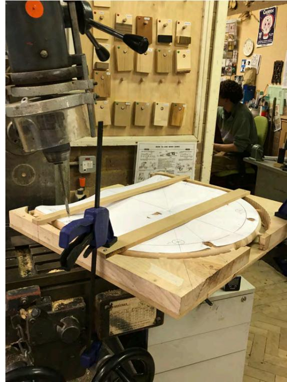
Front spindle hole drilling (20mm)
