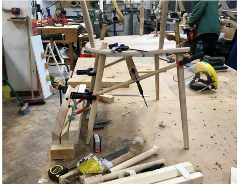
Side spindle angle test
