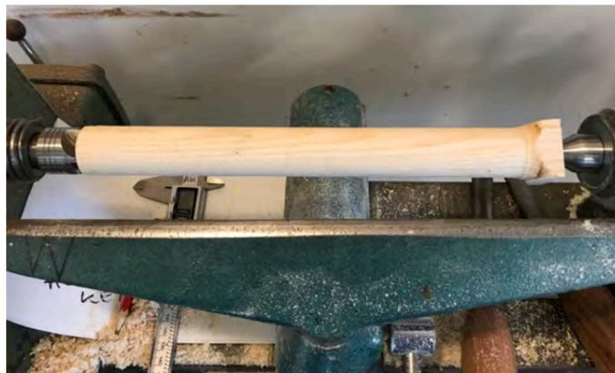
Spindle shaping on the lathe using a skew chisel & parting tool
