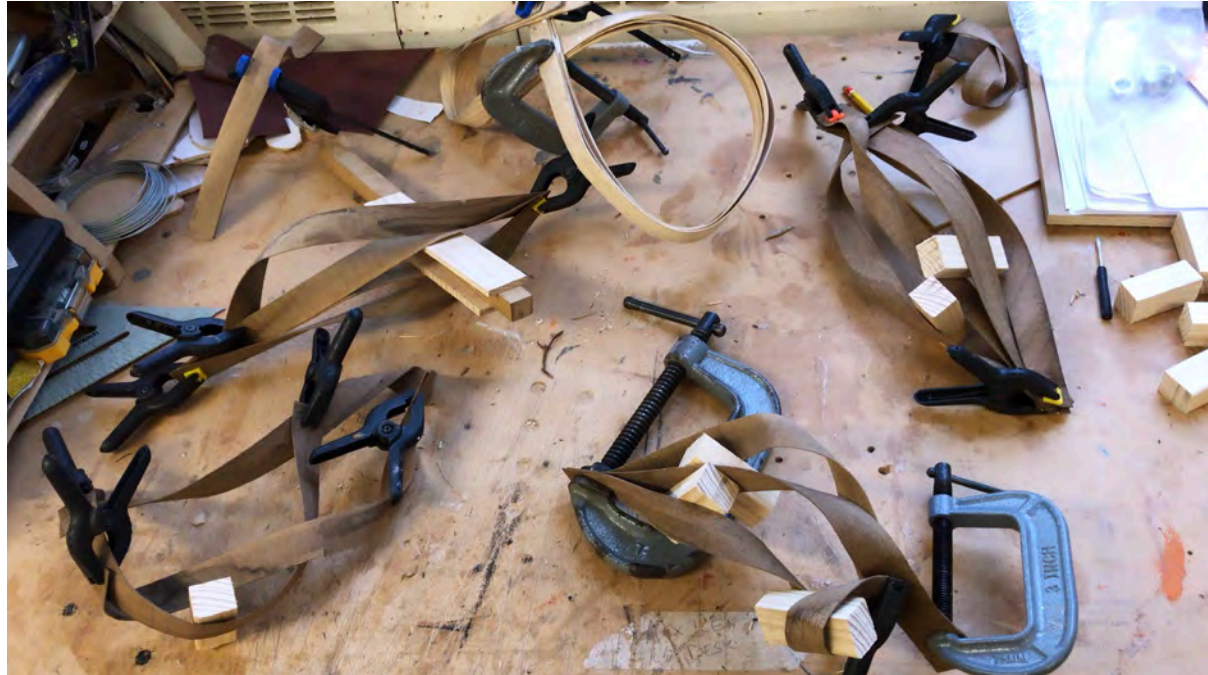
Free-hand walnut steam bending in the workshop Photography: Alex Key Date: Nov '19
