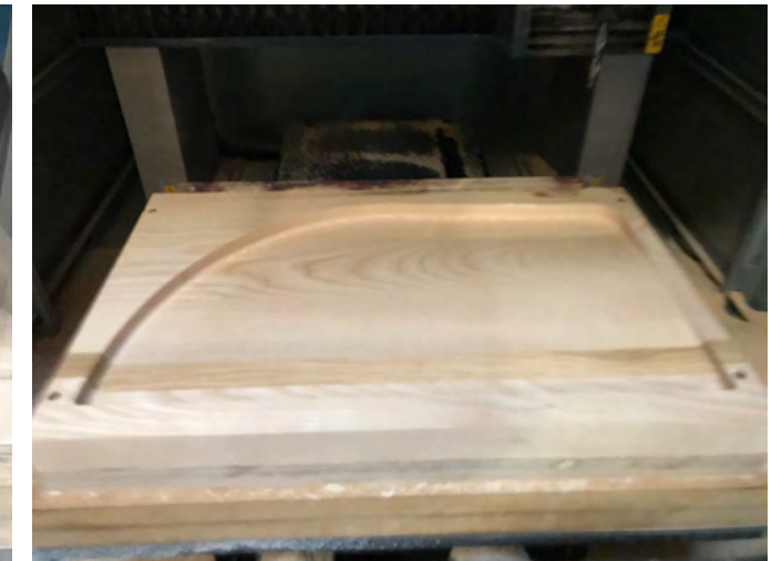
Seat bottom 3-axis milling Photography: Alex Key
