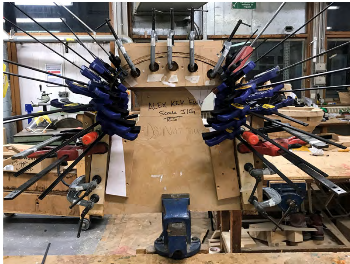
Ash back glue lamination clamp up Photography: Alex Key
