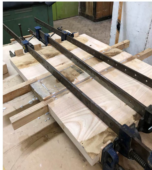
Seat blocks glued up in sash clamps 2 Photography: Alex Key
