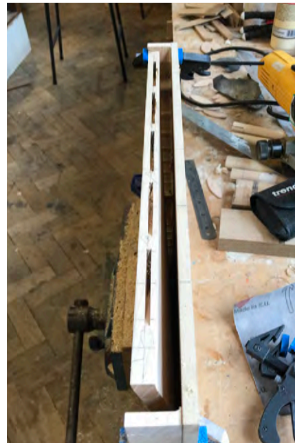
All the biscuit holes cut Photography: Alex Key
