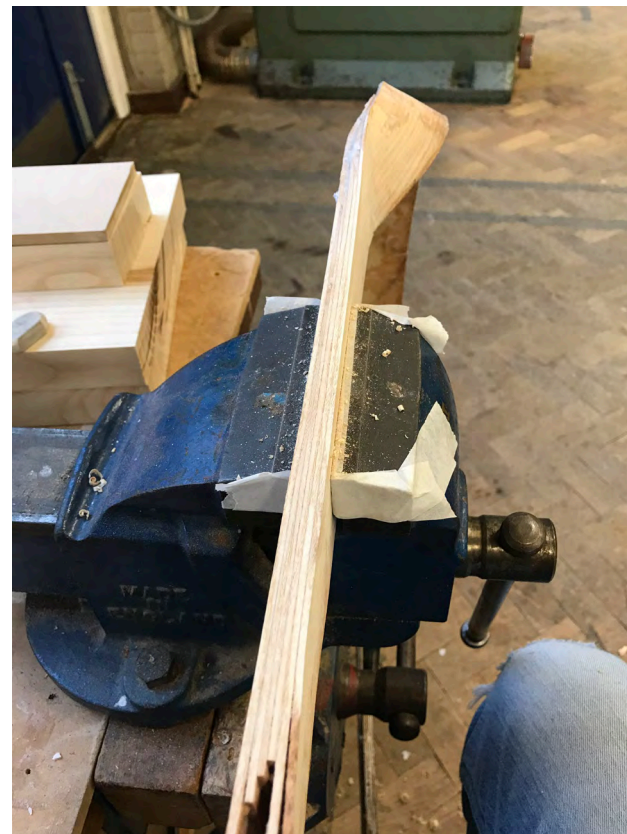
Ash back glue lamination clean up with a spokeshave Source: Alex Key
