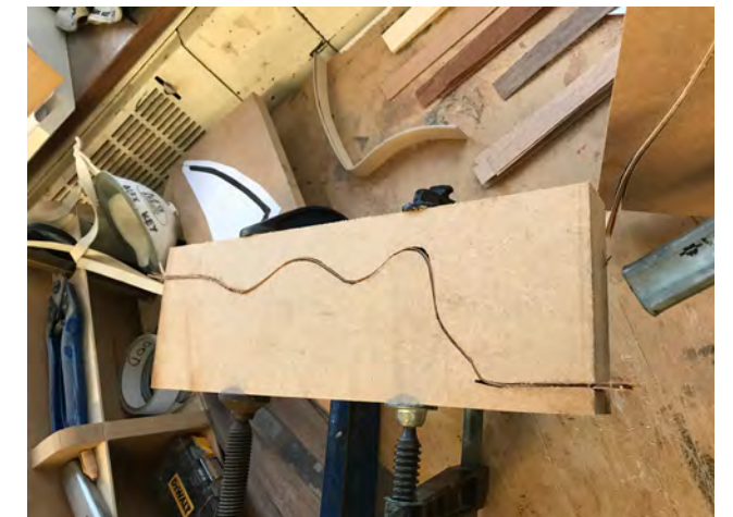
2-part compression JIG B - Oak strips Photography: Alex Key Date: Dec '19
