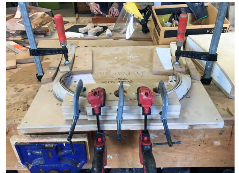
Ash strips in bending JIG 4 Photography: Alex Key
