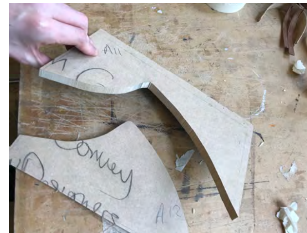
2-part compression JIG C Photography: Alex Key Date: Dec '19
