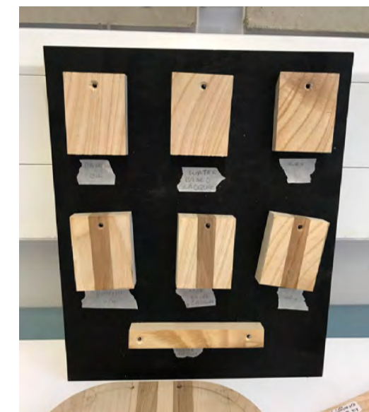
Finishes sample board - Water based lacquer, danish oil & wax Photography: Alex Key
