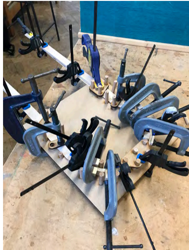
Sycamore back glue up A Photography: Alex Key Date: Jan '20
