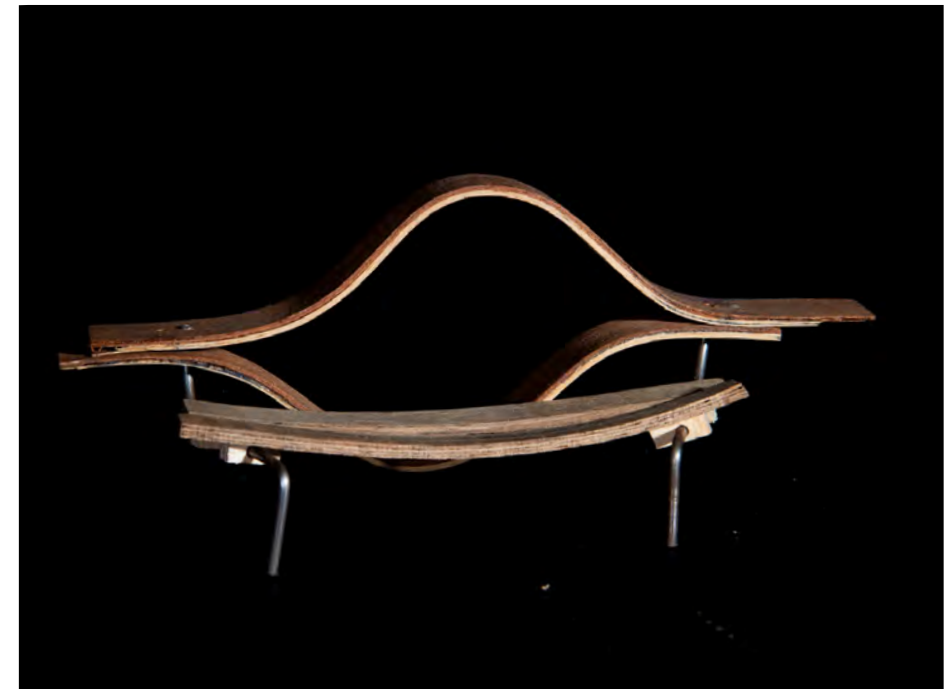
Initial bench model - Glue lamination tests Photography: Alex Key Date: Dec '19
