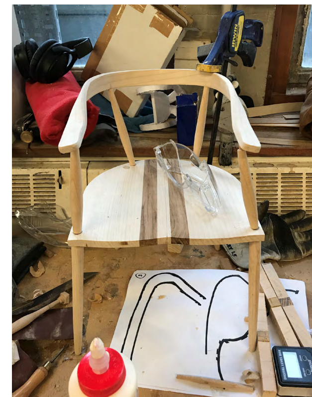
Spindles glue up Photography: Alex Key Date: Jan '20
