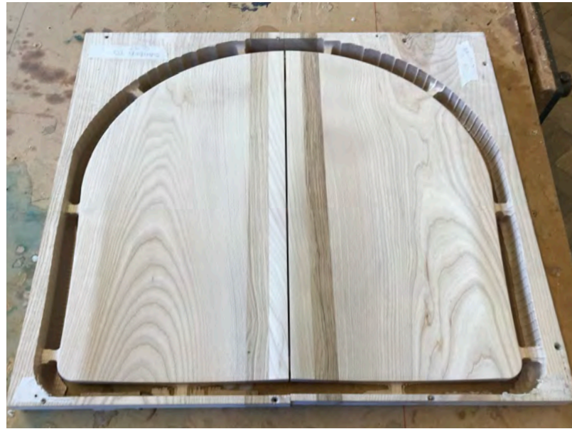
Milled seat halves 1 & 2 Photography: Alex Key
