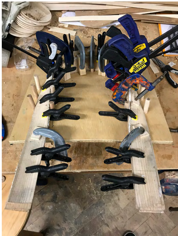
First glue lamination back test - Clamp up Photography: Alex Key Date: Dec '19
