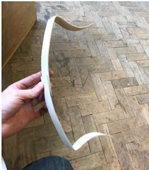
Glue laminations for initial chair model seat Photography: Alex Key Date: Dec '19
