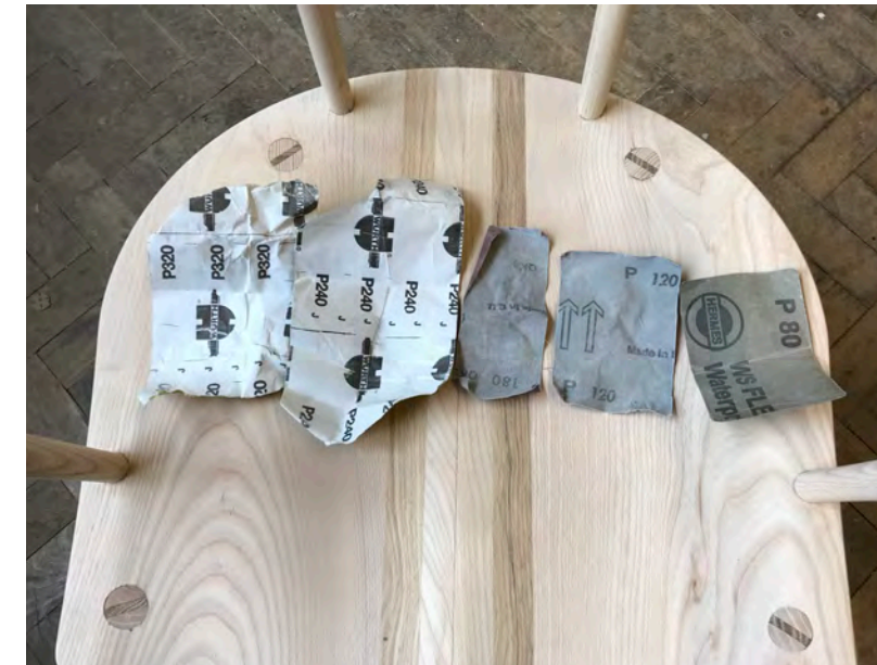
Sanding down - 80 to 320 grit Photography: Alex Key
