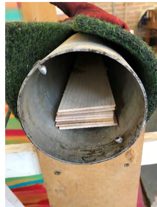
Ash strips in steam bender Photography: Alex Key
