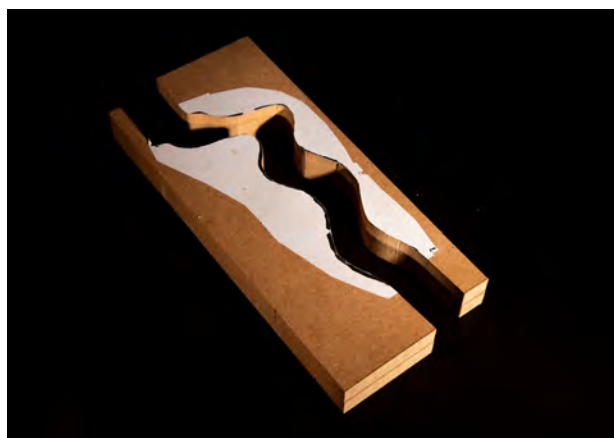
2-part compression JIG B Photography: Alex Key Date: Dec '19
