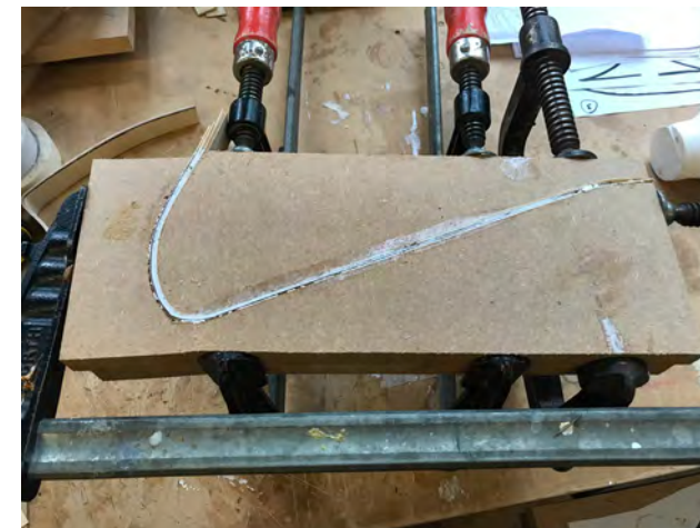
2-part compression JIG D - Oak strips Photography: Alex Key Date: Dec '19
