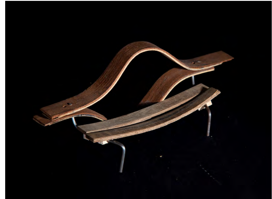
Initial bench model 1 - Glue lamination tests Photography: Alex Key Date: Dec '19
