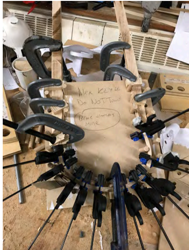
Sycamore back glue up B Photography: Alex Key Date: Jan '20
