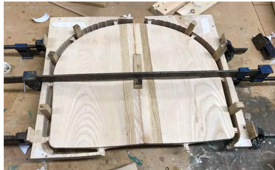
Milled seat glued together Photography: Alex Key
