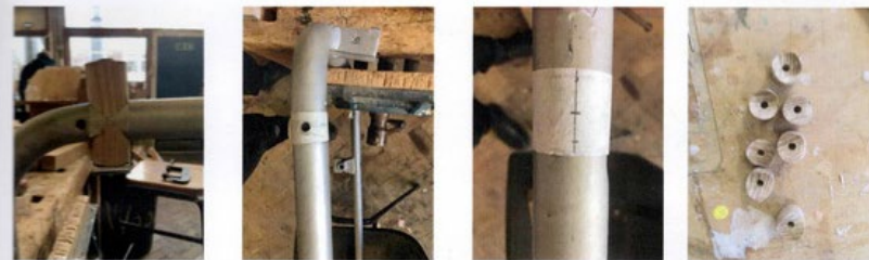
measured and drilled into the frame hard not to get the wood to split
