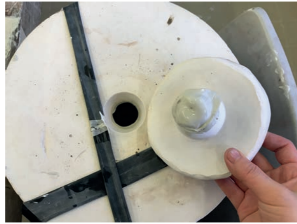
Remove the top mould at proper time
