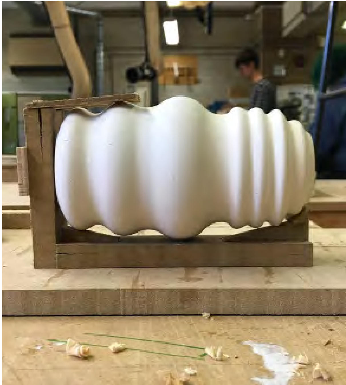
I made a wooden jig for my plaster object so that the object wouldn't rotate as it was being cut on the bandsaw - resulting in even slices of plaster.
