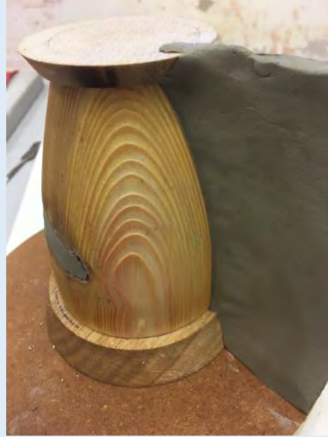
Casting a 4 Part mould to avoid undercuts.
