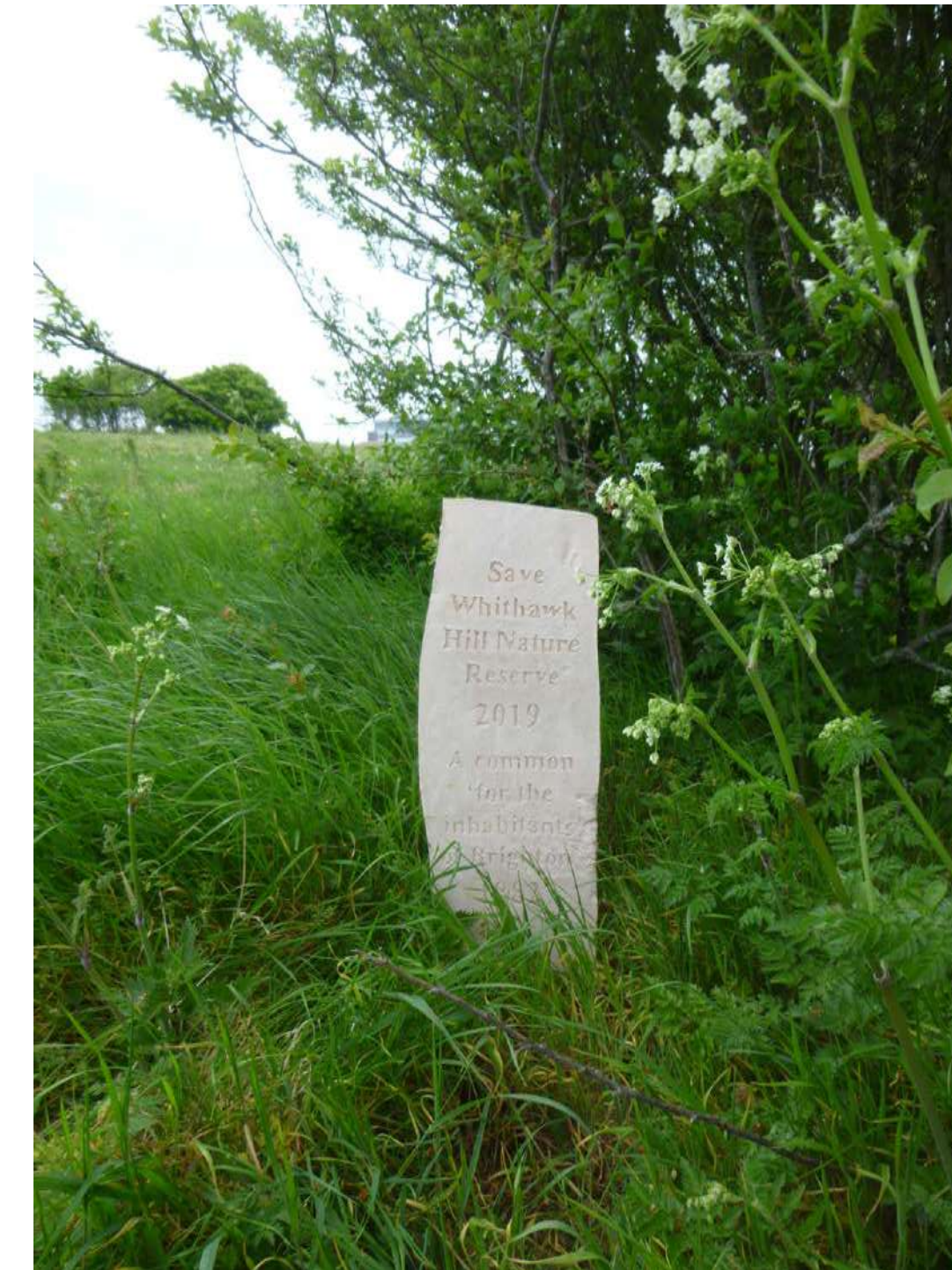
I took the test boundary stone up to Whitehawk hill as I wanted to see if its low firing would mean it would weather over the week.
