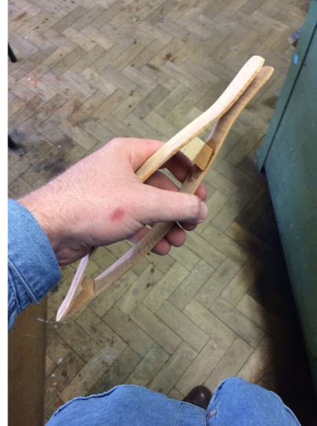
After initial tests with ash and Yew, I decided to go with Yew. Naturally a flexible wood, it worked perfectly.
