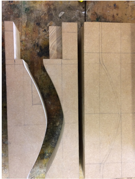
1. Former measured and band sawed
