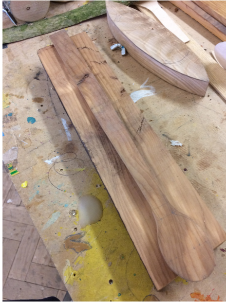
2. Spoon design marked up and cut using Yew.
