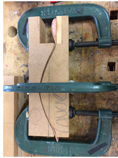
5. Each piece steamed for 15 minutes and bend for 4 days in former.
