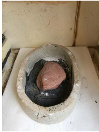
Second Firing Ramp- 60 Soak- 0 Temperature- 700
