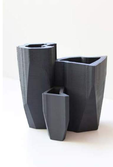
3D printing small models first before committing to laser cutting as this allowed me to see the work physically as opposed to just on a computer screen.
