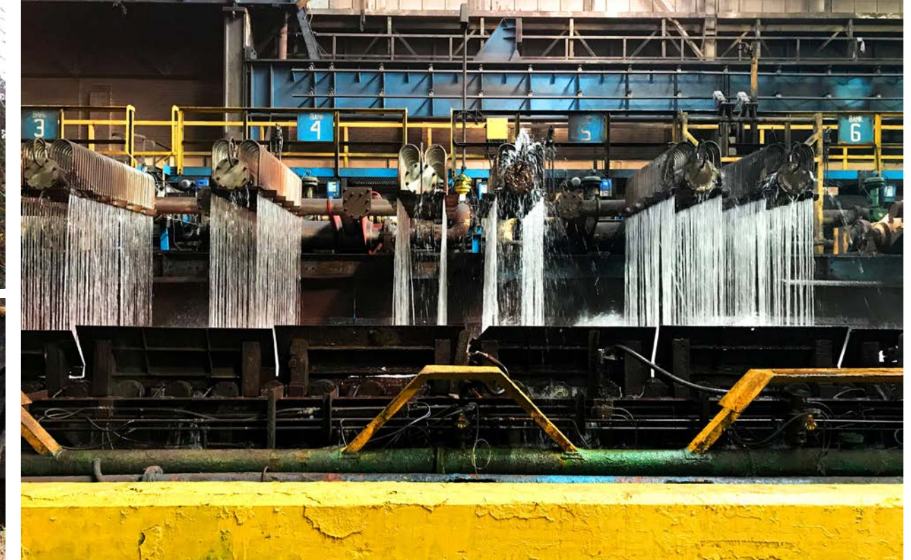
Water being used in the hot rolling mill to cool sheet steel down.
