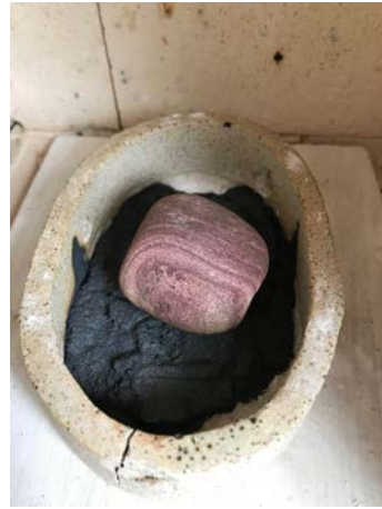
Fourth Firing Ramp- 60 Soak- 0 Temperature- 1260 (Stoneware)
