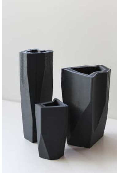
3D printing small models first before committing to laser cutting as this allowed me to see the work physically as opposed to just on a computer screen.
