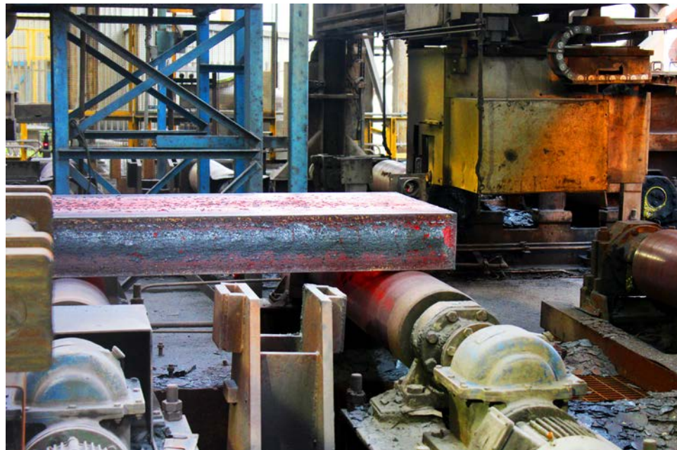
Finished steel slab being rolled out of part of the factory known as the heavy end of the steel production.
