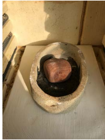
First Firing Ramp- 60 Soak- 0 Temperature- 400
