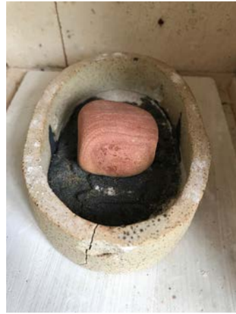
Third Firing Ramp- 60 Soak- 0 Temperature- 1000
