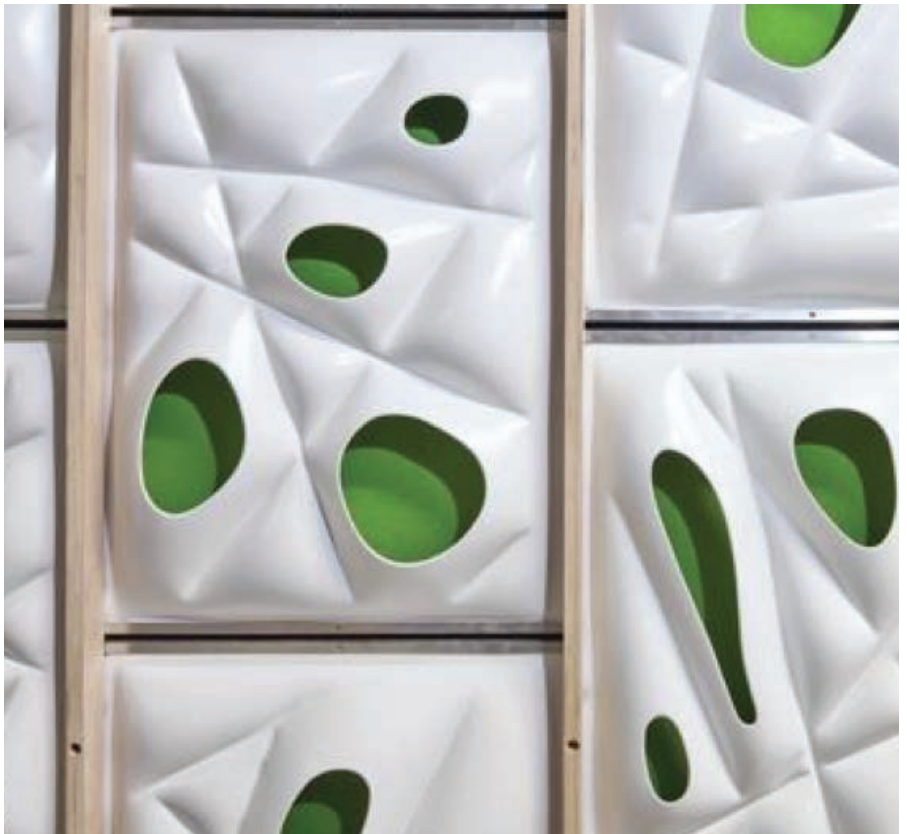
Vacuum Forming and complexity through analog variability
