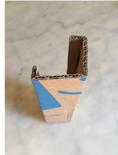
Edges are folded in here to give an illusion of being more solid and weighty. This design looks more considered as well as being more sturdy
