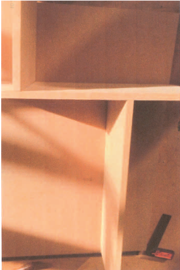
I used wood filler to cover up any joints and end grain of the MDF as I didnt want the piece to look like wood but wanted to create the illusion of it having a zinc/lead look.
