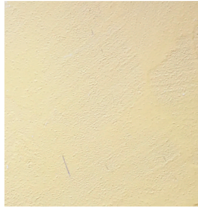
Tadelakt tests, textures and finishes with ochre pigment.
