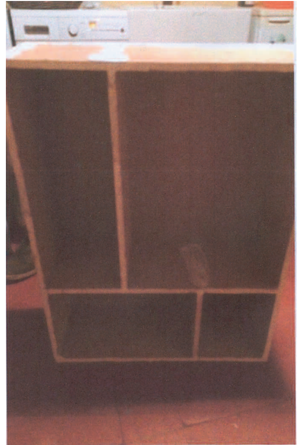
I used wood filler to cover up any joints and end grain of the MDF as I didnt want the piece to look like wood but wanted to create the illusion of it having a zinc/lead look.
