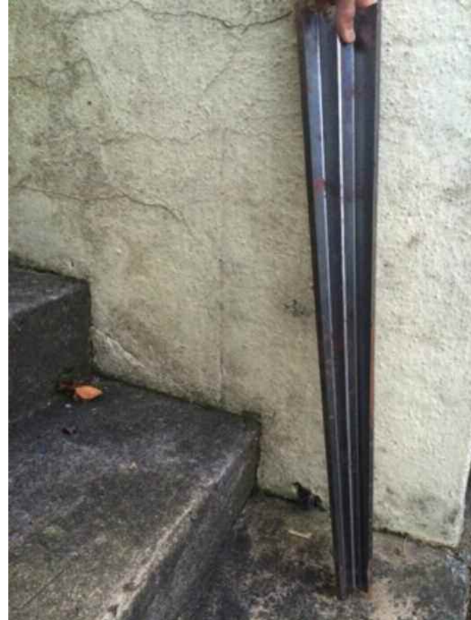
Steel leg prototype. I feel the leg looks too ultra modern in raw steel so I will be considering powder coating or chemical blackening for a more subtle and grounded look.
