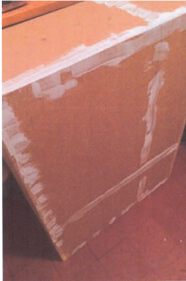
I used wood filler to cover up any joints and end grain of the MDF as I didnt want the piece to look like wood but wanted to create the illusion of it having a zinc/lead look.
