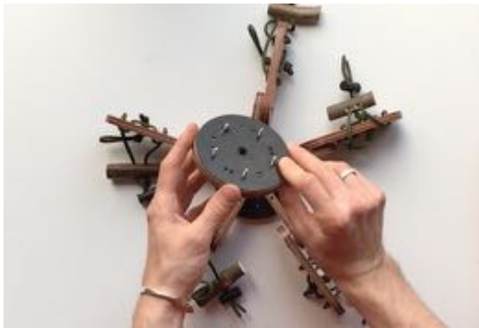
Step 4: Add the top plate to the assembly making sure that each screw locates properly in the arm holes.
