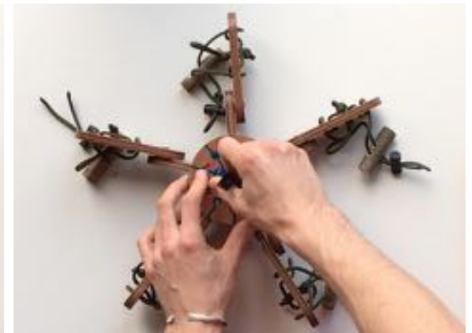
Step 5: Finally, add the quick release scrower to the assembly. Close the quick release when loose and wind clockwise to a tighten enough. * Avoid overtightening the quick release.
