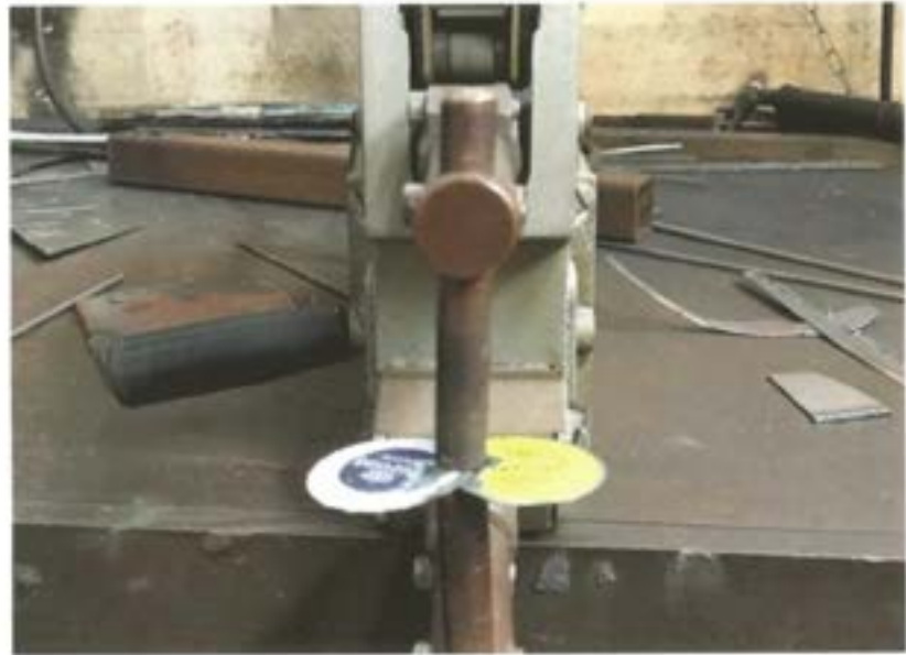
Welding them together
