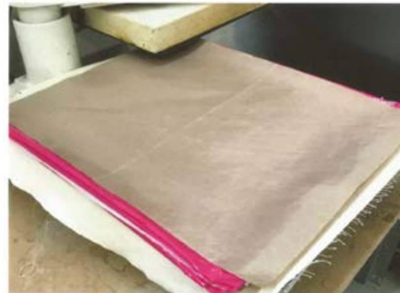
Placing the bags on the heating press
