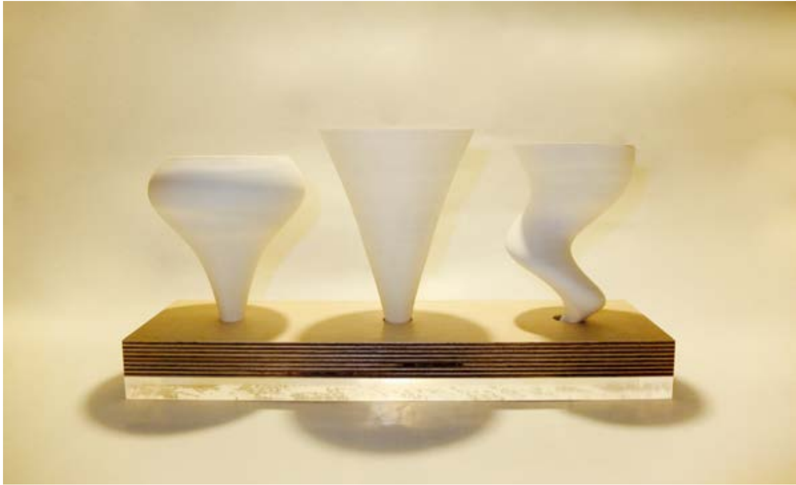
The final three cones and the holder. The cones being 3D printed and the holder made from 18mm Ply and 15mm clear acrylic.
