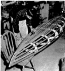
All edges of the completed hull frame must be planed and sanded smooth so that the canvas cover will not wear at any spots. This is important.
