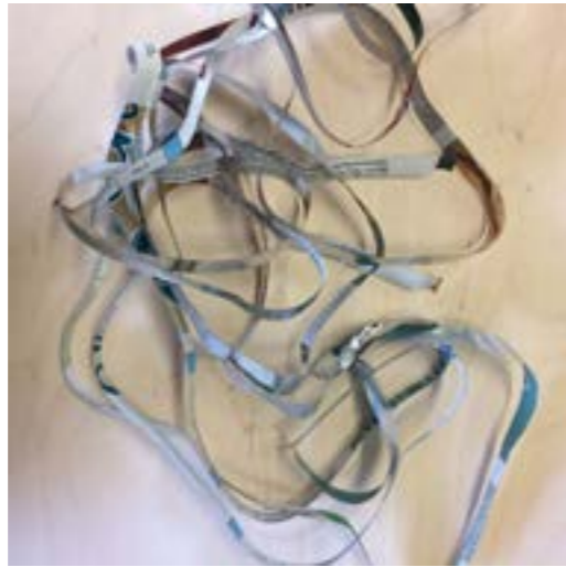
Colour samples - Nepal is a colourful and vibrant place and using colour was appropriate. Recycled plastic sting - this initial test was too thick and rigid to fit through the holes in the plywood.
