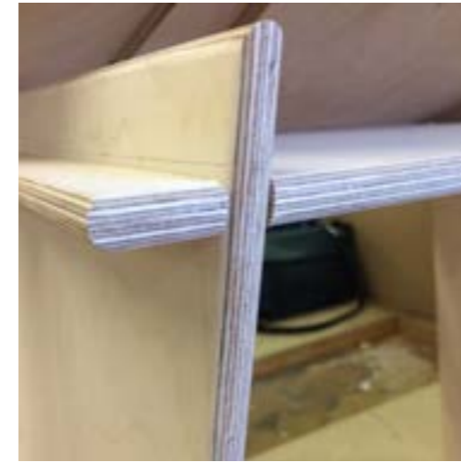
Plywood mock up - it was important to test the design in the intended material - to test strength and aesthetics of the plywood.
