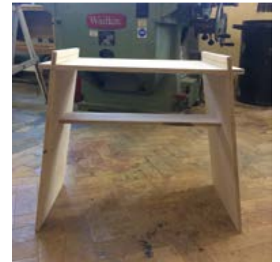
Plywood mock up - it was important to test the design in the intended material - to test strength and aesthetics of the plywood.
