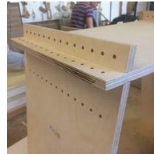
Plywood mock up - it was important to test the design in the intended material - to test strength and aesthetics of the plywood.
