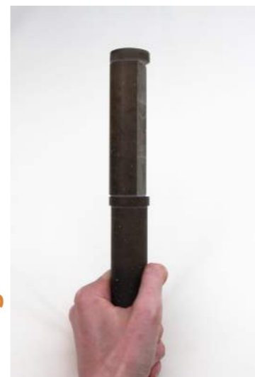
Milling a flat face for bristles
