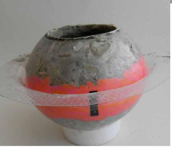
I again chose to vacuum form the mold in two parts, but this time leaving out an opening at the top so I would be able to press the concrete into the form allowing as thin a wall as possible. Keeping the delicate feel of the concrete.
