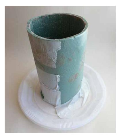
Making the molds for these time capsules proved much more difficult than my earlier pieces. I decided to vacuum form the molds in two parts so I could easily take the set concrete out, however by using a plastic mold the excess water in the concrete mix isn't able to evaporate out and so unless the concrete is completely set there is the danger that the piece could break.
