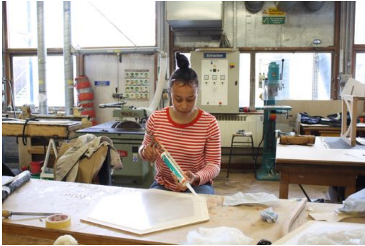
The inner frosted acrylic screens were each hand cut out using the band saw and then attached to the frame using a silicone adhesive.
