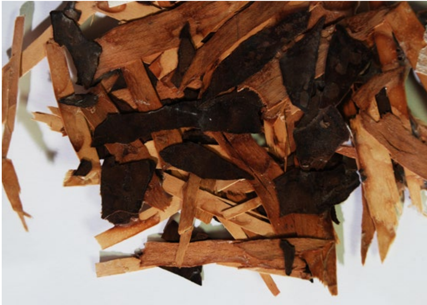
WOOD CHIPPING + PVA GLUE, COMPRESSED UNDER A BOOK PRESS.
